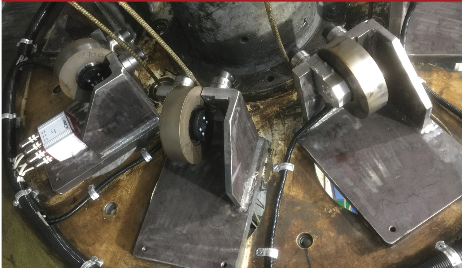
▲ Force measuring rollers and amplifier module
